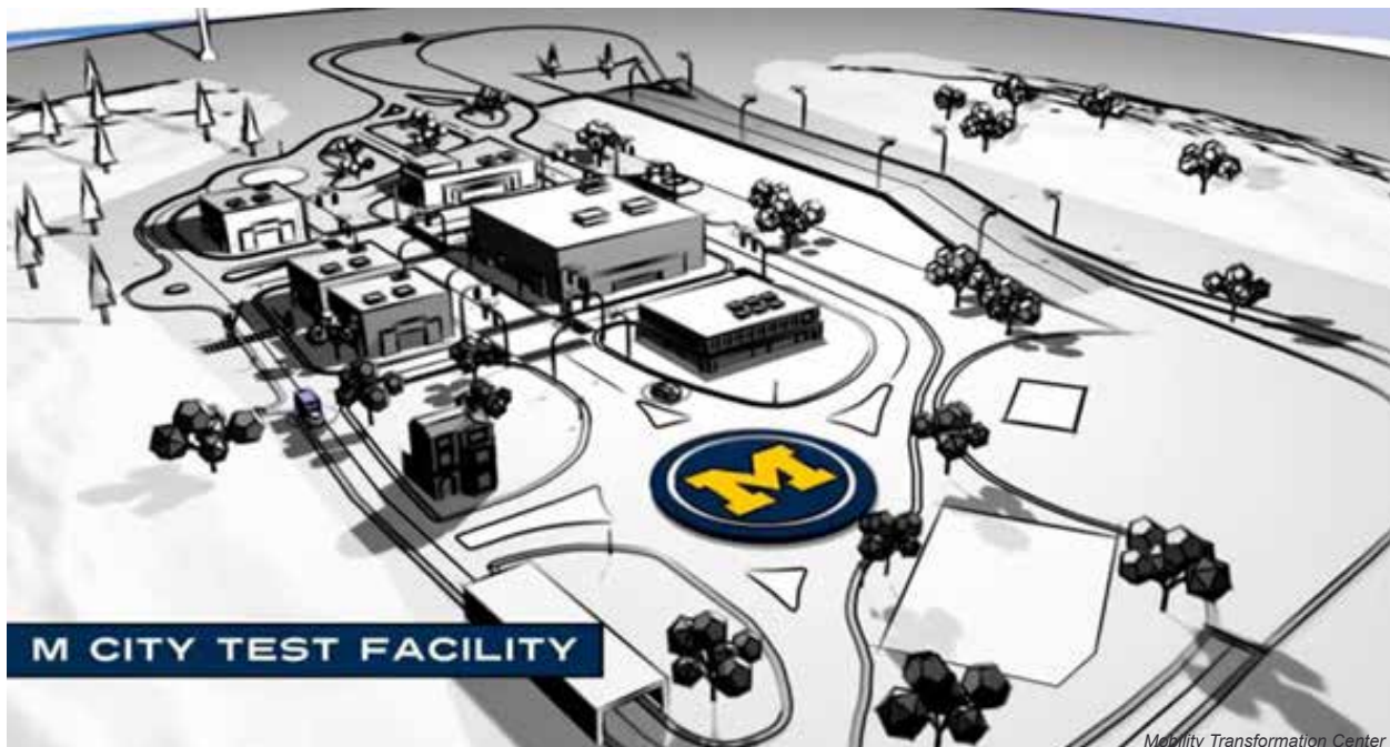
M City is a full-scale simulated city designed and built to create an off-road testing environment for autonomous vehicles. It includes approximately five lane-miles of roads with intersections, traffic signs and signals, sidewalks, benches, simulated buildings, street lights, and obstacles such as construction barriers for closed testing by auto manufacturers. The facility opened in July 2015.
